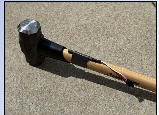
Hammer Switch mounted on Top of Sledgehammer
